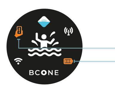
Low Pool Unit Battery Alert – Both mobile device icon and battery icon are simultaneously on it indicates low Pool Unit battery.
